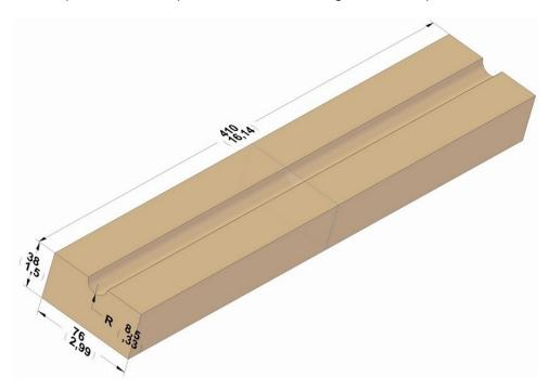
2. Then glue two by two pieces together, so that in the center you will get circular opening 17mm in diameter, just like it is shown on the pictures.
