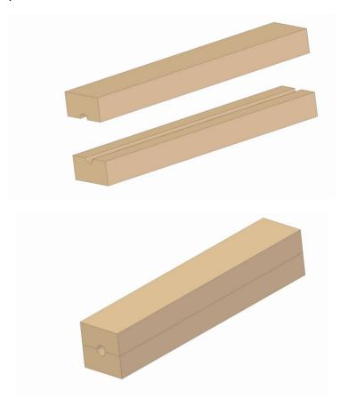
3. While you are waiting for glue to dry, you can make the template of an external contour for Post Segments. This template will help to make flawless and identical turnings of each Post Segment. When you make sure that the glue is dry, put the subassembly into the wise and make the first Post Segment using template and a chisel.
