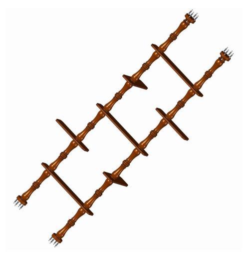
Flower pot stand consists of Post segments, which you are going to make on the lathe and pull the steel bar through them. Shelves for the plants are placed between these Post segments. This assembly then needs to be fixed with the screws onto the ceiling and to the floor.
