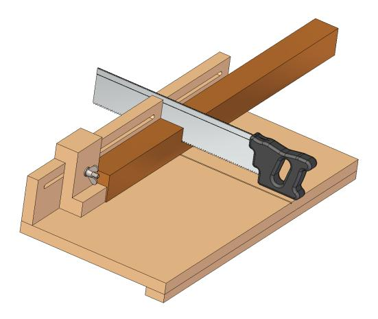
On this page, we present a jig that allows you to cut slats//laths quickly and easily into same-length pieces using a hand saw.
