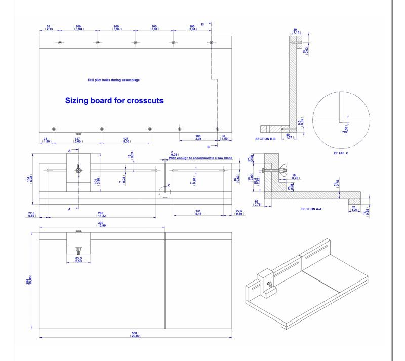
You will make fences by cutting the wood part from the picture in two pieces. Be careful to leave enough space between them for the saw blade, during the fastening process to the base.
